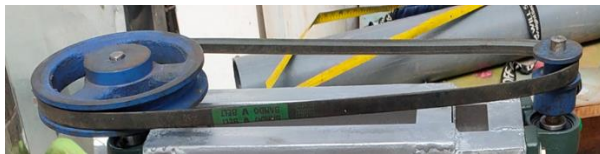
Gambar 5. V-belt tipe B 51
