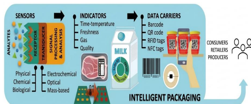
Figure 2. Intelligent Packaging Mechanism (Versino et al., 2023)
