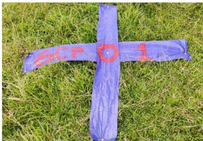
Gambar 4. Pemasangan premark Ground Control Point (GCP)
