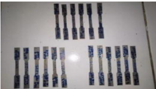
Gambar 3. Sampel Uji Tarik
