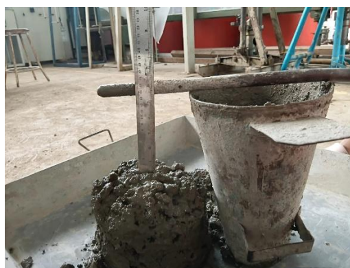
Gbr. 2. Pengujian Slump
